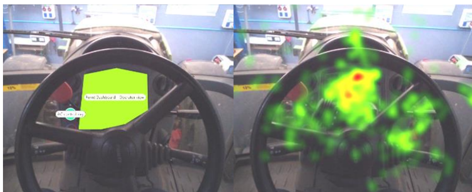
Fig. 12. AOI1 the notification panel and AC rotary switch with the heatmap generated
