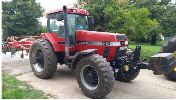
Fig. 7. CASE 7210 with attached cultivating tool
