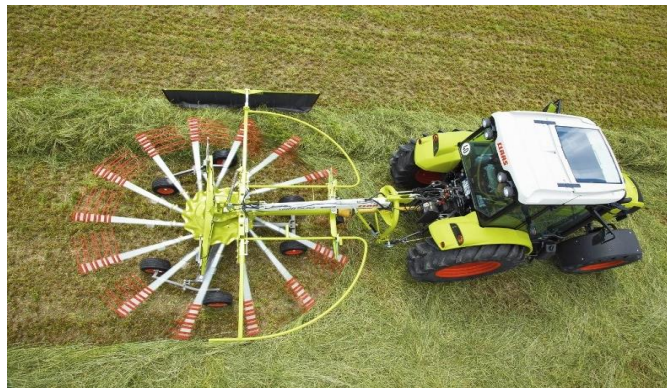
Fig. 3. ARES 567 ATZ tractor with CLAAS LINER 450T used for windrowing
